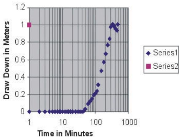
Fig. 8: Shows the results of Constant Discharge Test (CDT) and the changes in the water level Reading done for well No. 10. June 8, 20104
