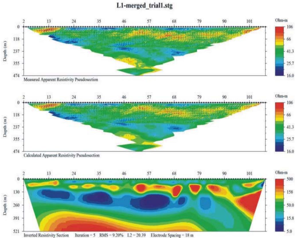
Fig. 9: Inverted resistivity section for two-dimensional for profile -1
