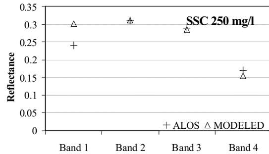
Fig. 7: Comparison of modeled and ALOS/AVNIR reflectance data
