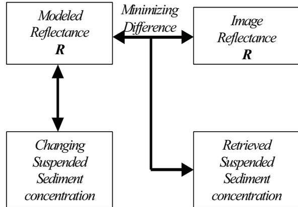
Fig. 5: Concept diagram of model inversion technique
