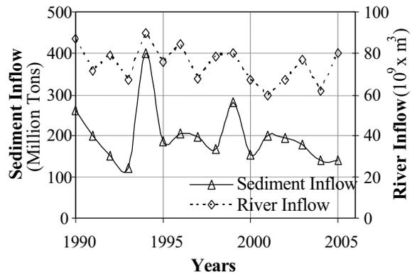
Fig. 1: Annual sediment load computed from hydrograph survey
