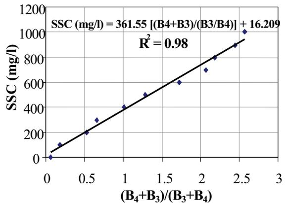
Fig. 3: Relationship between SSC and developed reflectance model
