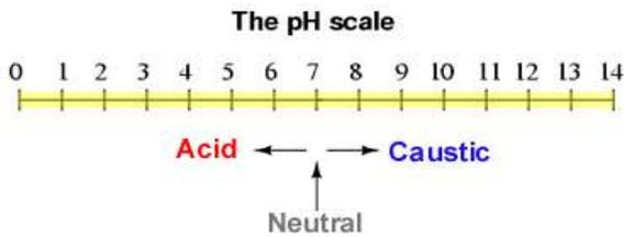
Fig. 2: The scale of pH of different solutions.
