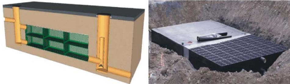
Fig. 7: Underground infiltration blocks – scheme [14],CR [18]
