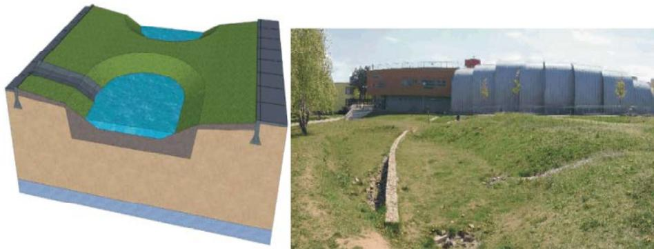
Fig. 2: Swale infiltration –left scheme [14], right Kohoutovice, Brno, CR
