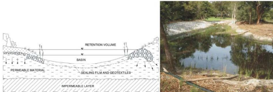
Fig. 6: The basin with permeable slopes [17]
