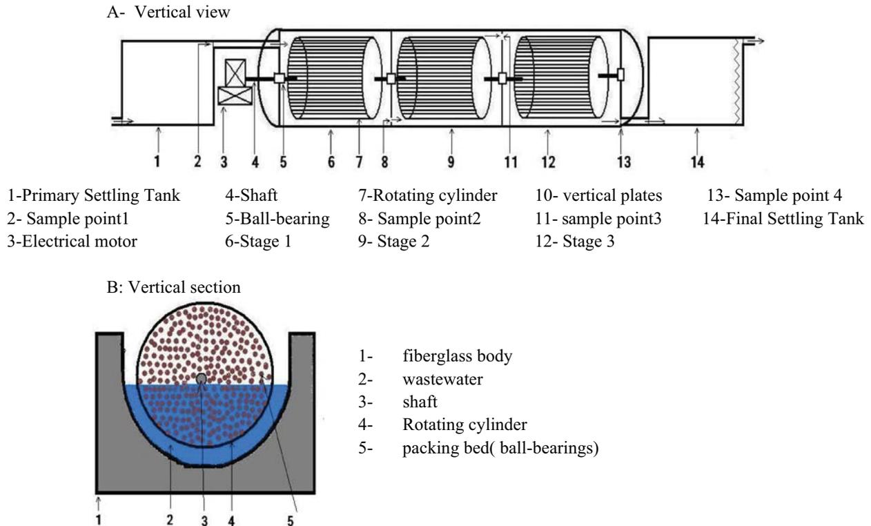
Fig. 3: Schematic representation of the RBCp pilot plant
