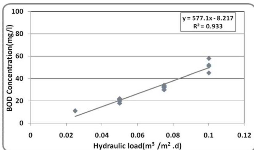
Fig. 8: Relationship between effluent BOD concentration and Hydraulic load
