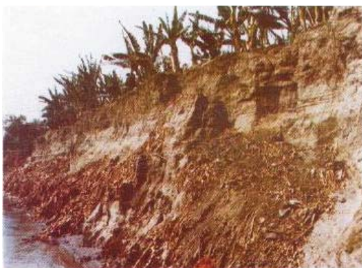
Photo 1: Composite land failure as a result of toe material removes (hydraulic factors)
